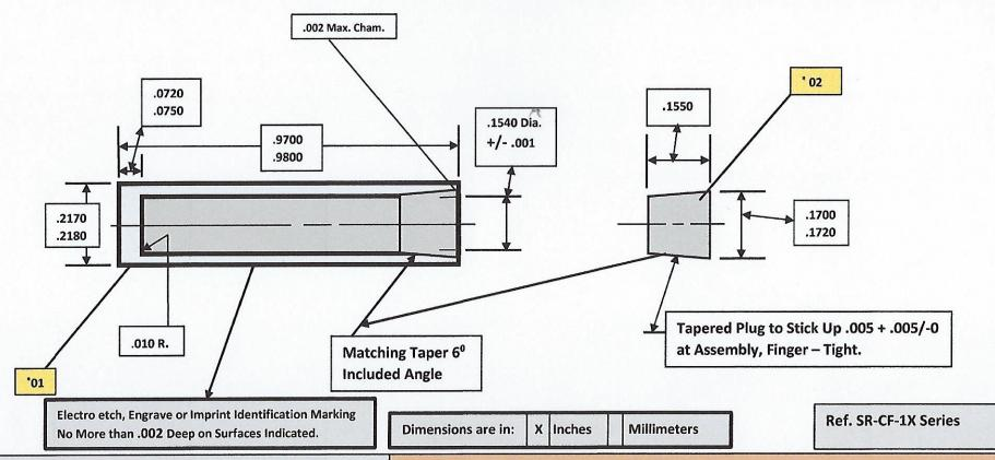
Notes: 1. Break All Corners .010 - .020 unless otherwise specified. FRONTIER TECHNOLOGY CORPORATION 2. Press Plug Flush with Container Top, TIG Weld. (Minimum 0.030 Weld XENIA, OHIO, U.S.A. Penetration, Measured Along Joint).
